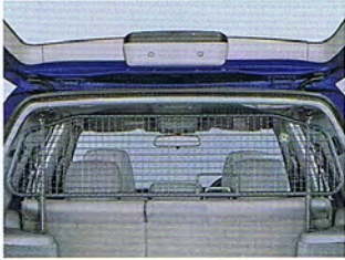
41. Dog guard (G/M) Separates cargo room from passenger area, applicable for ISO FIX child seat.
