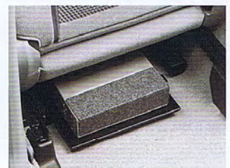
66. CD changer tray Attachment required to mount CD CHG or Navi unit.
