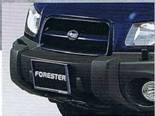
22. Front bumper guard Helps protect bumper and front of engine from brush and debris.
