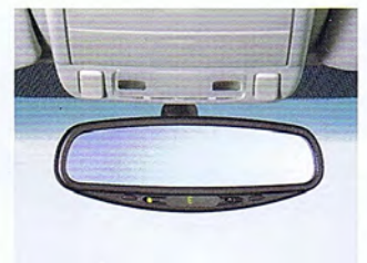
73. Auto-dimming compass mirror Includes electronic compass. Mirror darkens when headlights are detected from the rear of the vehicle.
