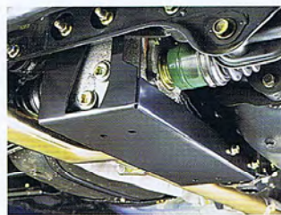
29. Differential protector Helps protect rear differential from rocks and logs.
